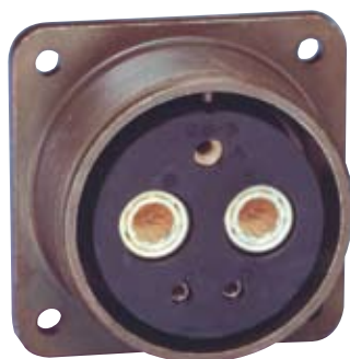
Amphe-Power 5015 connector with insert pattern 28-5 with (2) size 4 RADSOK® sockets and standard contacts.
