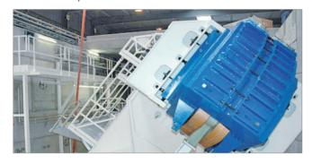
The gantry rotates around the patient's bed and is responsible for beam guidance. Central factors in this respect are the splitting and control of the particle beam to ensure that it can be focused on the treatment target in the body as precisely as possible. The mobility of the installation increases the requirements placed on the radio frequency connectors since they must also provide a high level of flexibility to withstand repeated bending without any adverse effect on performance.
