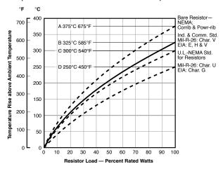
Fig. 2: Approximate hot spot temperature rise of a resistor in free air for various specifications.
