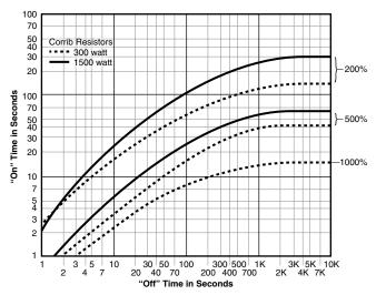
Fig.12: Percent of Continuous Duty Rating for Pulse Operation of  $\mbox{CORRIB}^{\circledast},$  Corrugated Ribbon Resistors.
