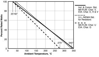
Fig. 4: Derating of Resistors for High Ambient Temperatures.
