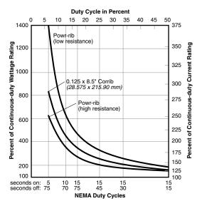
Fig. 8: Percent of Continuous Duty Rating for Resistors for Typical NEMA Duty Cycles.
