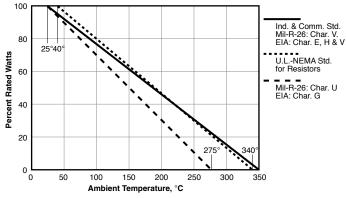
Fig. 3: Derating for ambient temperature.
