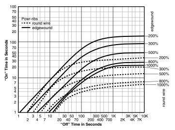
Fig. 13: Percent of Continuous Duty Rating for Pulse Operation of Powr-Rib $^{\circledast},$  Bare Resistors
