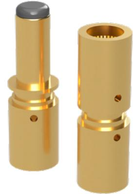
This can be improved further by manufacturing contacts from high conductivity material. The standard contact material used by Positronic is copper alloy. However, the use of Tellurium Copper increases the conductivity and reduces the temperature rise. Tellurium copper contacts are a standard option across the Panther family, allowing engineers to take advantage of this high-performance material.
